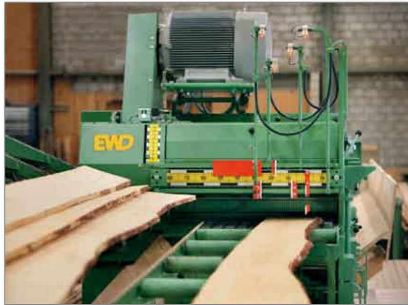
Clear pointers indicate the position of the saw heads and the pickers at the machine. Perfect board alignment by means of moveable laser lines.
