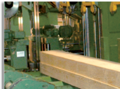
Centering system for guiding of the cants in front of the bandsaws
