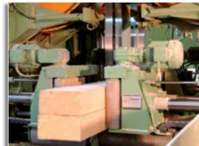
Centering system for guiding of the sawn lumber behind the bandsaws
