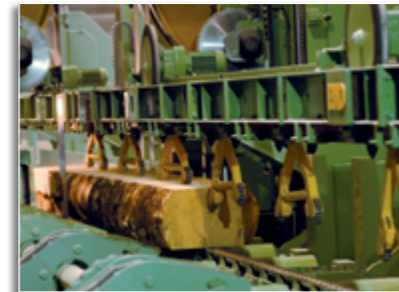
Logs and cants are held between top and bottom hold and feed elements
