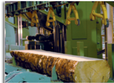
Alignment arms for the positioning of logs and 2-sided cants
