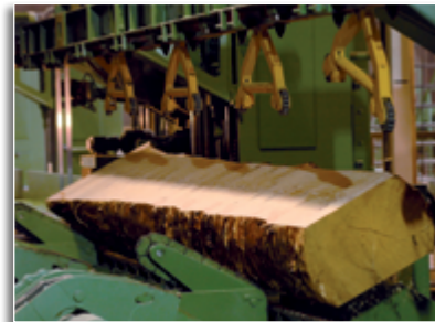
Chain arms for turning of logs and cants
