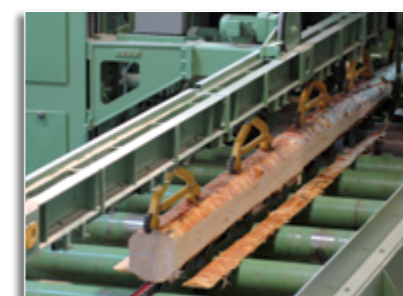
1. Sawing of slabs
