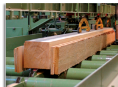
5. Sawing secondary side boards
