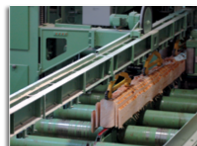
2. Sawing side boards
