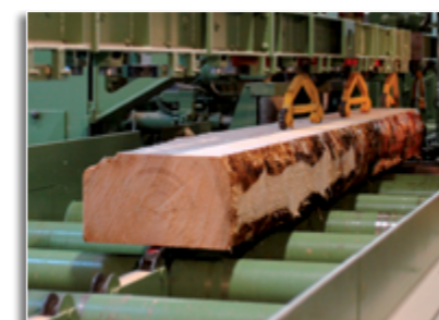
4. Sawing slabs secondary breakdown
