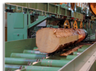
2. Sawing slabs primary breakdown
