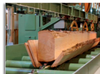
3. Sawing primary side boards
